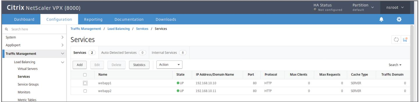
This screen shows that during the first step of the process webapp1 has been taken offline. This is the time when the backend software can be updated.
