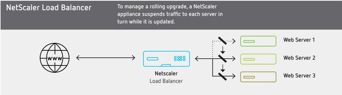
Let's see how Ansible can be used to take each server offline in turn to update a service, without causing any disruption to customers. While the update made here is trivial, the same process can be used to perform series of much more complex updates.
